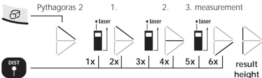
The 2nd measurement takes place with automatic Min/Max function.
