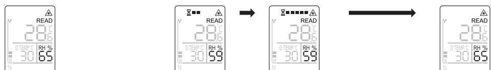
Relative humidity is automatically determined and displayed during the measurement process.
